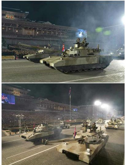
http://1.lt's based on a T-72, this can be seen by the central mounted drivers pos, rear circular fan cover, exhaust and roadwheels, some people say it's a T-62, but they are wrong. There is an extra roadwheel thrown in the mix so it has a slight extension to the hull https://t.co/g672zpV92O
